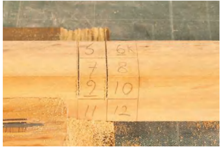
▲ Pic.8 Starting to make the cuts that will create the voids
